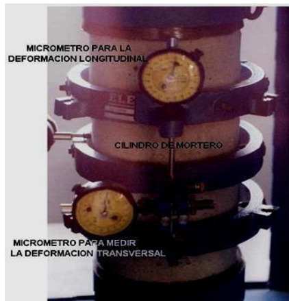
Figure 2. Arrangement of equipment for measuring modulus of elasticity in cylinders.
