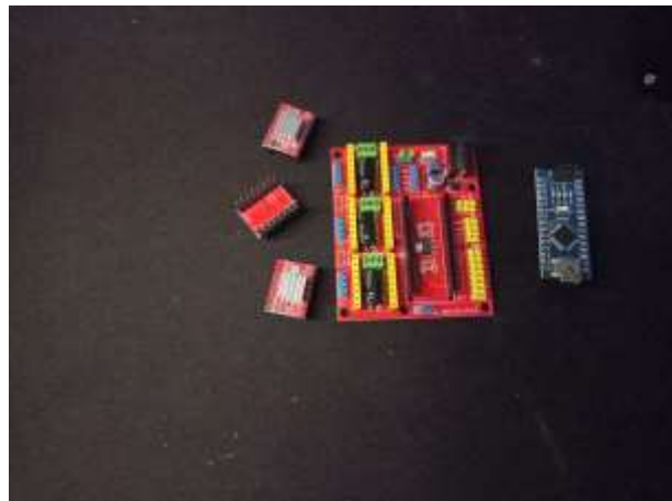
Figure 15. Top view of the motor control board and the Arduino NANO board.
