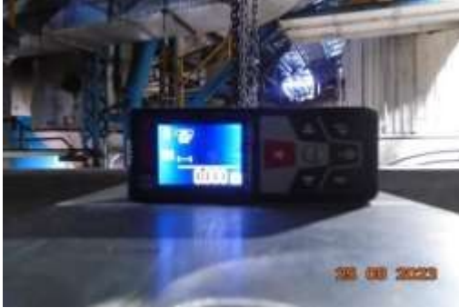
Figure 3. Test using a digital level and laser. Source: Author's own work.
