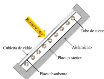
Figure 1. Parts of a flat plate collector.
