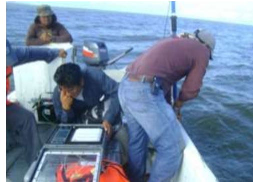
Figure 7. Figure showing the bathymetric survey (measurement of sea depths to determine the topography of the seabed) with the appropriate specialized equipment.
