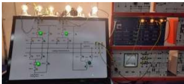
Figure 19. Line 1 and bar 1 energized in the physical prototype.
