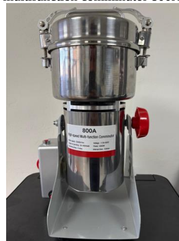
Figure 1. Bagasse fiber size reduction mill.
