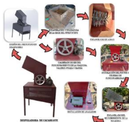
Figure 7. Representative schematic of the peanut peeling machine prototype. Source: Own elaboration, 2025.
