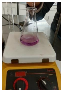
Figure 2. Sample with black eriochrome indicator T. Source: Own elaboration.
