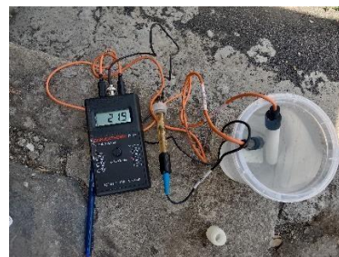
Figure 1. Measurement of TDS, g/L Temperature °C and pH. Source: Own elaboration.
