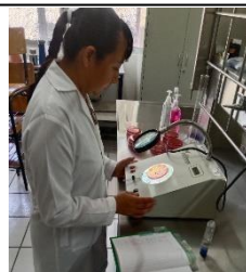
Figure 10. CFU count with the colony counter, Felisa. Source: Own elaboration.
