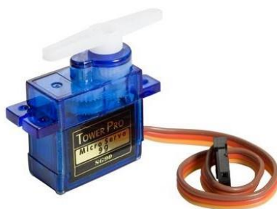
Figure 4. sg90 servomotor used in hexapod robot.
