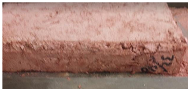
Figure 9. Mix 1 brick, crumbled after compression test.
