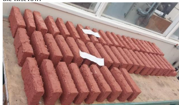
Figure 2. Bricks of Mix 1 and Mix 3.
