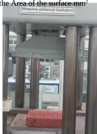
Figure 7. Sample brick of Mix 4 in Universal Machine.
