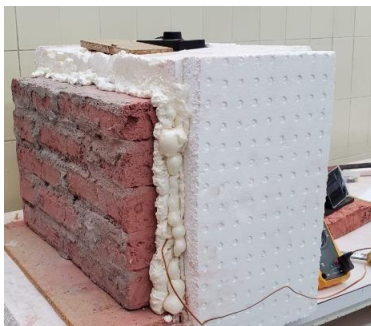
Figure 8. Arrangement for temperature difference measurement.
