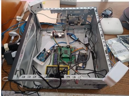
Figure 2. Physical Architecture of the Remote-Lab.
