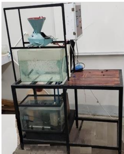
Figure 9. Automated system for hormone treatment of tilapia fry.
