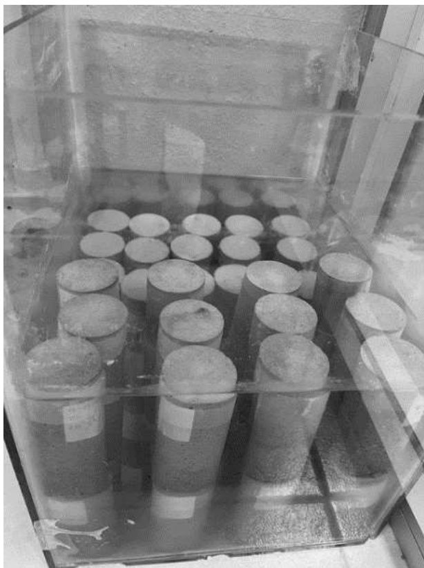
Figure 2. Curing of specimens at 7, 14 and 28 days Note: Taken by authors.
