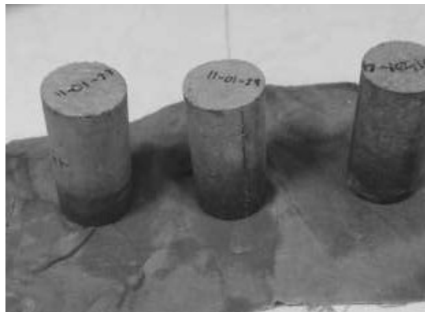
Figure 3. Cylinders just removed from the storage tank to prevent moisture loss.
