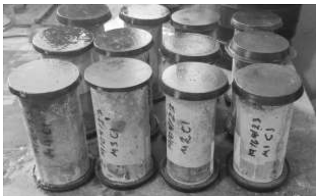
Figure 5. Specimens with 75% sulfur and 25% sand mortar pitch. Note: Taken by authors
