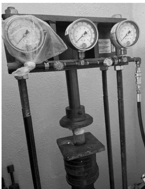
Figure 6. Compressive strength test. Note: Taken by authors The results are recorded in a logbook.
