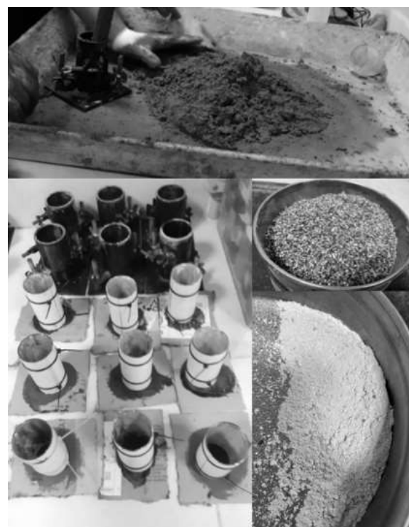
Figure 1. Mixture preparation and experimental cylinders Note: Taken by authors.
