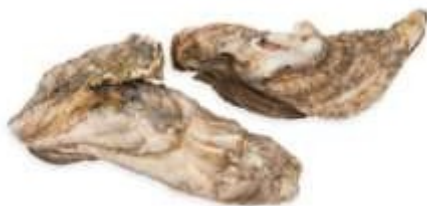
Figure 1. Unprocessed oyster shell in fine aggregate. Figure 1 shows the oyster shells with a first wash with water and bicarbonate to remove residual edible matter.
