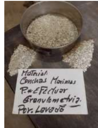
Figure 2. Oyster shells transformed into washed fine aggregate.
