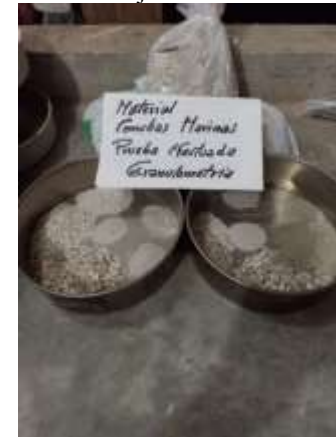
Figure 3. Washed oyster shells transformed into fine aggregate and granulometric test performed.
